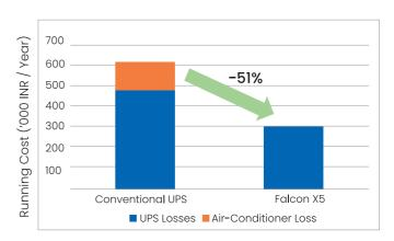
Calculation Conditions: Total annual running cost at Rs.7/kWh and 30% (100 kW) load
